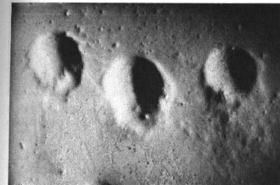
Fig. 78. Raindrop imprints with elliptical impact craters, because of the oblique direction of falling drops. The rim of the impact crater is broken on one side. Laboratory experiment. (After Reineck 1955a)
