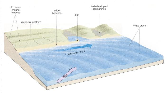
**FIGURE 15.1** *Emergent* coastline features. An emergent coastline is caused by sea-level lowering, the land rising, or both. Emergence causes tidal flats and coastal wetlands to expand, wave-cut terraces are exposed to view, deltas prograde at faster rates, and wide stable beaches develop.
