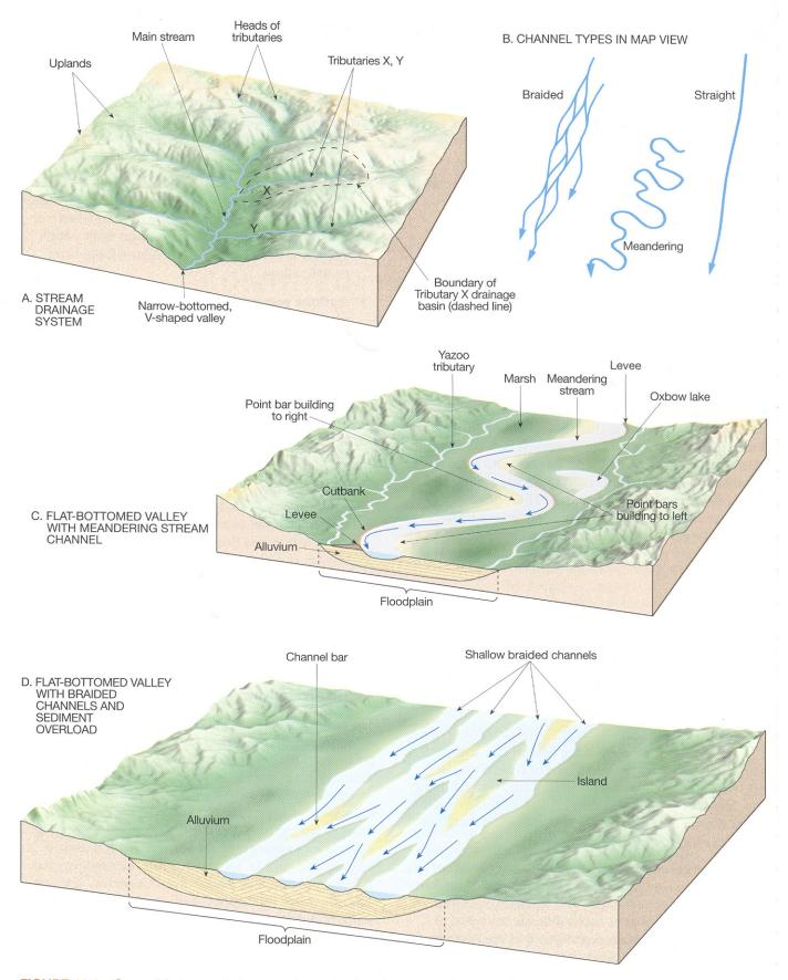
**FIGURE 11.1** General features of stream drainage basins, streams, and stream channels. Arrows indicate current flow in main stream channels. **A.** Features of a stream drainage basin. **B.** Stream channel types as observed in map view. **C.** Features of a meandering stream valley. **D.** Features of a typical braided stream. Braided streams develop in sediment-choked streams.
