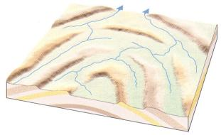
**Annular:** Long channels form a pattern of concentric circles connected by short radial channels. Develops on eroded domes or folds with resistant and nonresistant rock types.
