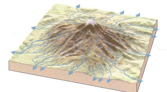
Radial: Channels radiate outward like spokes of a wheel from a high point.
