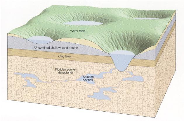
FIGURE 12.7 Geologic cross section showing groundwater distribution in strata underlying the Tampa, Florida, area.
