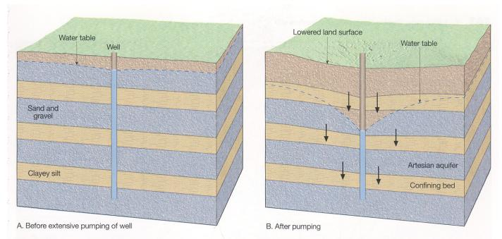
**FIGURE 12.9** Before (**A**) and after (**B**) extensive pumping of a well. Note in **B** the lowering of the waterpressure surface, compaction of confining beds between the aquifers, and resulting subsidence of land surface. Arrows indicate the direction of compaction caused by the downward force of gravity, after the opposing water pressure was reduced by excessive withdrawal (discharge) of groundwater from the well.
