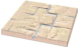
**Rectangular:** Channels have right-angle bends developed along perpendicular sets of rock fractures or joints.
