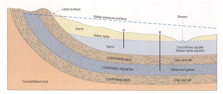
**FIGURE 12.10** Geologic cross section illustrating an unconfined (water-table) aquifer and a confined aquifer. Vertical scale is exaggerated.
