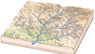
**Dendritic:** Irregular pattern of channels that branch like a tree. Develops on flat lying or homogeneous rock.
