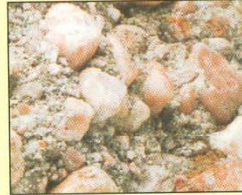
Conglomerate: made mostly of rounded gravel and sand grains (usually quartz grains)
