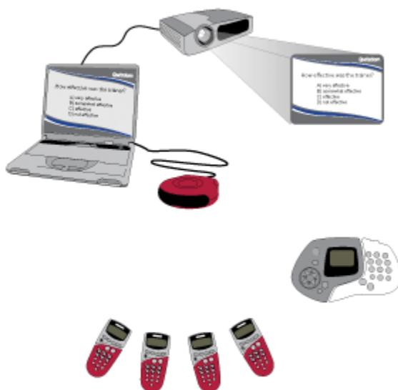
Qwizdom's **Response System** includes a host, which plugs into the instructor's laptop or desktop USB drive, teacher remote, and student remotes. The host transmits a radio frequency which allows communication with the instructor's computer, the teacher remote, and student remote. This RF IEEE standard system helps insure robust, conflict-free operation and supports up to 1,000 remotes at one time.
