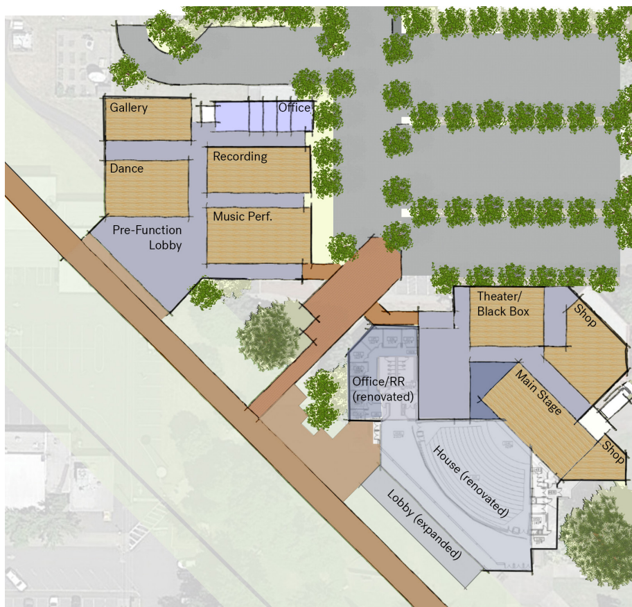
Figure 77: Conceptual layout of a new Arts facility, on the current site of a cluster of modular classrooms. Goals include: separation of louder uses (shops) from programs such as music and dance, as well as aligning active entries along the open space.
